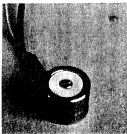
(a) Force coil (b) Sensing device Fig. 3: Main unit of the 5-axis motion sensor
